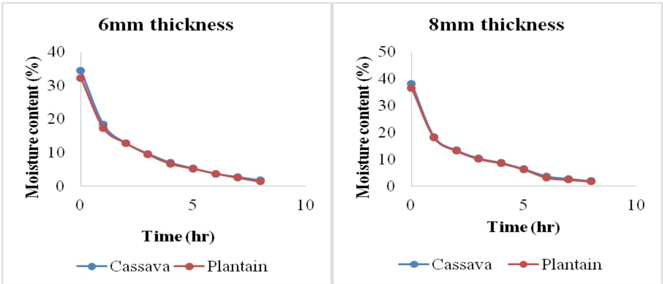
Fig. 1: Graphs of moisture content against time for tray drying
