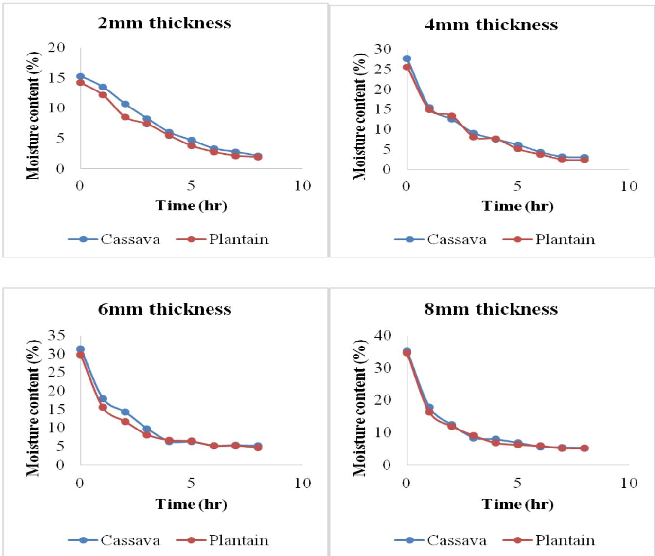
Fig. 2: Graphs of moisture content against time for sun drying
